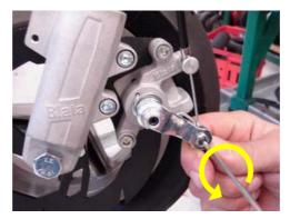
unscrew the screw 312.018.00 and remove the brake pads and the brake pad spring from the
